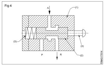
Working principle of 3 port 2 position valve:
