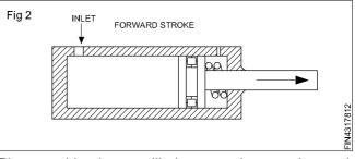
Piston and load move till piston reaches to other end. At the end there is no further space for piston to move, hence piston and load movement stops. (Fig 2)
