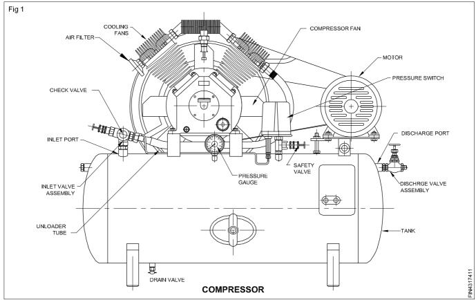
The following are the main parts of an air compressor.
