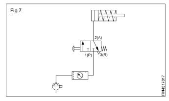
When compressor is switched on compressed air is available up to input port "1" (Fig 8)
