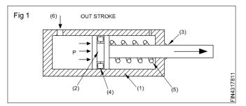
Main parts of single acting cylinder are listed as follows:
