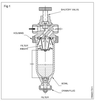
Fitter, regulator, lubricator (FRL) assemblies are prepackaged or modular assemblies of air filters, pressure regulators, and gauges. Air leaving a compressor is hot, dirty, and wet and can cause damage to equipment and tools if it is not filtered.
