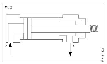
Piston movement will stop if air does not exhaust.
