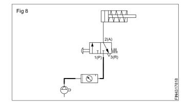
When push button is pressed, direction of air changes due to valve shift. Piston moves forward. (Fig 9)
