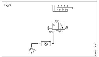
Push button is when released piston returns back. (Fig 8)
