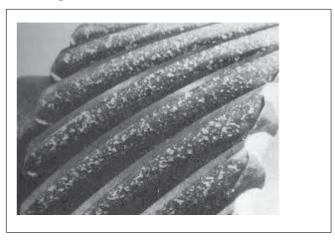
Causes: Surface irregularities, misalignment of gears.
