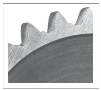
Cause: Wear in progress, in a dequate lubricant film
