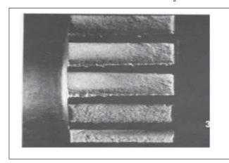
**Plastic flow:** Cold working of tooth surfaces caused by high contact stress.
