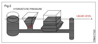
Therefore the higher pressure in any of the container will force the liquid to flow to the next container until the pressure on both the sides are equalised.
