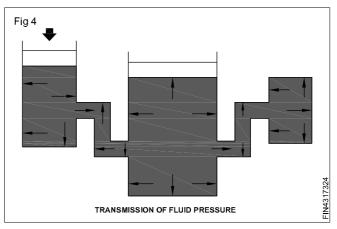
Thus if small amount of pressure is exerted on a smaller piston as shown in Fig 5, the higher force can be attained at the larger piston, since the pressure is equally applied on larger area.
