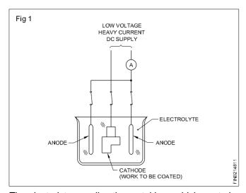
The electrolyte supplies the metal ions which are to be deposited on to the components (cathode). The anodes may be soluble and made of the same metal to be plated on the component surface i.e. nickel, copper or zinc.
