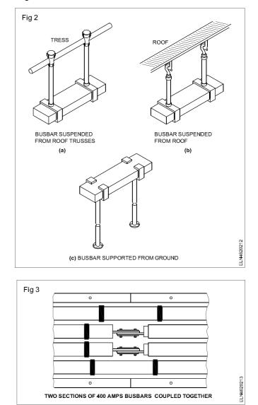
The standard rating of bus-bar are 100, 200, 400, 600, 800, 1200, 1600, 2000, 2400 and 3600 ampere with rated voltage of 500V. These bus-bars also available for indoor or outdoor use as point to point feeders or as plug-in take off points for power. These bus-bars are used in generating stations, sub stations, in metal industry and textile industry. These bus-bars are also used in multi storied flats to facilitate connection to various stories from the mains by
