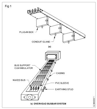
This bus-bar system is sometimes referred to as bus way or bus duct.
