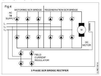
If the SCRs were gated with a phase angle of zero degrees, then the drive function as a rectifier which feeds the full rectified rated DC supply to the motor and by varying the firing angle to the SCRs, a variable DC supply is applied to the motor.
