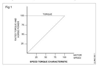
Generally, a fixed field supply is provided in these DC drives. As the torque is constant (which describes a load type) over the speed range, the motor output horse power is proportional to the speed. The motor characteristics of this drive are in Fig 1.
