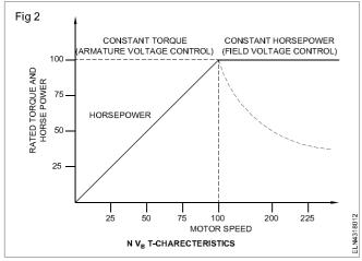
In most instances the shunt field winding is excited, with a constant - level voltage from the controller . The SCR (silicon controller rectifier), also known as thyristor, which converts the alternating current (AC) of the power source to variable DC output which is applied to the armature of a DC motor. Speed control is achieved by regulating the armature voltage to the motor.
