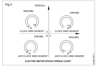
**Quadrant I:** Driving or motoring forward accelerating quadrant with positive speed and torque
