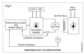
**Rectifier Bridge:** The power component of a controlled DC drive is a full wave bridge rectifier which can be driven by three phase or single phase supply. As mentioned above the number of thyristor may vary depends on the supply voltage.
