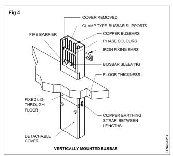
Recommended current density for a copper bus-bar which is not enclosed should not exceed 165A/sqcm and for aluminium 118A/sqcm.
