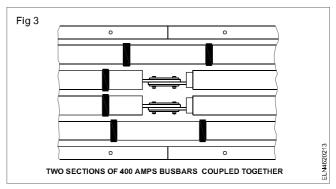
The standard rating of bus-bar are 100, 200, 400, 600, 800, 1200, 1600, 2000, 2400 and 3600 ampere with rated voltage of 500V. These bus-bars also available for indoor or outdoor use as point to point feeders or as plug-in take off points for power. These bus-bars are used in generating stations, sub stations, in metal industry and textile industry. These bus-bars are also used in multi storied flats to facilitate connection to various stories from the mains by
