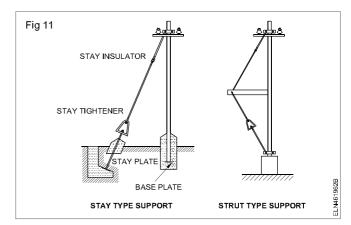
One end of the stay is fixed at the top of the pole and its other end is grouted in the concrete foundation.
