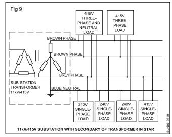
The star point is earthed to an earth electrode sunk into the ground below the substation, and from this point is taken the fourth conductor, the neutral. Loads connected between phases are fed at 415V, and those fed between one phase and neutral at 240V.
