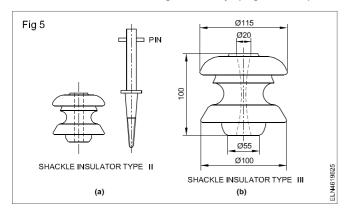
But now a days, they are frequency used for low voltage distribution lines. Such insulators can be used either in horizontal position or in a vertical position. They can be directly fix to the pole with a bolt or to the cross arm. Fig 6 shows a shackle insulator fixed to the pole. The conductor in the groove is fixed with a soft binding wire.
