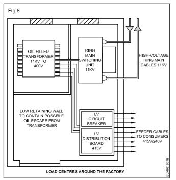
These outgoing circuits are usually protected by circuit breakers in a distribution board.
