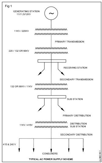
The ordinary power plant capacity and generating voltage may be 11KV, 11.5 KV, 12KV or 13KV. But economically. It is good to step up the produced voltage from (11KV, 11.5KV or 12KV) to 132KV, 220KV, 400KV or 500KV or greater (in some countries, up to 1500KV) by step up transformer (power transformer).
