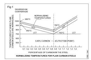
Soaking is holding at the heating temperature for 5 mts./ 10 mm of thickness for carbon steels.
