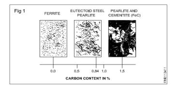
The structure of steel becomes visible when a piece of the metal is broken. The exact grain size and structure can be seen through a microscope. Steel is classified according to its structure.
