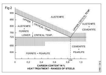
If steel is heated, a change in its structure commences from 723°C. The new structure formed is called 'AUS-TENITE'. Austenite is non-magnetic. If the hot steel is cooled slowly, the old structure is retained and it will have fine grains which makes it easily machinable.
