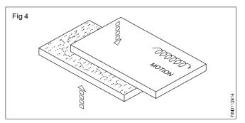
Observe the high spots on the plates X and Y and remove by scrapping. (Fig 5)
