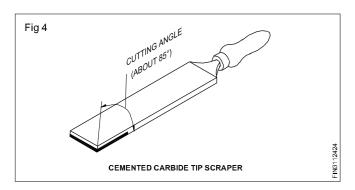
The cutting edges sharpened by grinding should be honed. Honing removes grinding marks and provides keen cutting edges.
