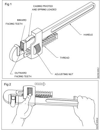
Once the jaws are adjusted, the spring loading keeps them in contact with the work, and the toggle action causes the hardened serrations to bite into the work.
