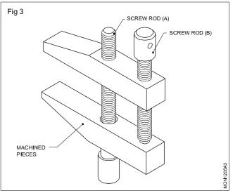
The head of the screw-rod (B) is provided with a hole through which a cylindrical pin may be passed for tightening purposes. The toolmaker's clamps are for holding a previously machined work which is flat and parallel.
