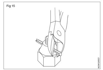
They are also used for spreading the cotter pin.
