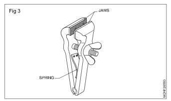
Hand vices are used for gripping screws, rivets, keys, small drills and other similar objects which are too small to be conveniently held in the bench vice. A hand vice is made in various shapes and sizes. The length varies from 125 to 150 mm and the jaw width from 40 to 44 mm. The jaws can be opened and closed using the wing nut on the screw that is fastened to one leg, and passes through the other.
