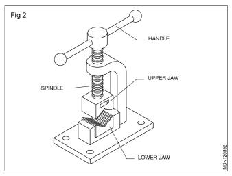
A Pipe vice is used for holding round sections of metal, and pipes. In this vice, the screw is vertical and movable. The jaw works vertically.
