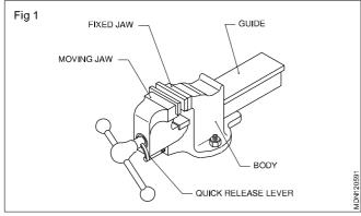
A quick releasing vice is similar to an ordinary bench vice but the opening of the movable jaw is done by using a trigger (lever). If the trigger at the front of the movable jaw Fixed jaw, movable jaw, hard jaws, spindle, handle, boxnut and spring are the parts of vice.
