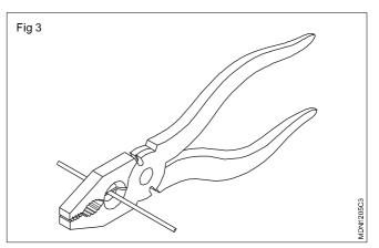
Two joint cutters are provided for cutting or shearing off steel wires (Fig 4)
