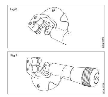
before every use lubricate the centre bolt threads, with graphite - based lubricant
