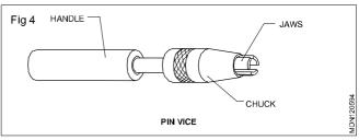
The pin vice is used for holding small diameter jobs. It consists of a handle and a small collet chuck at one end. The chuck carries a set of jaws which are operated by turning the handle.
