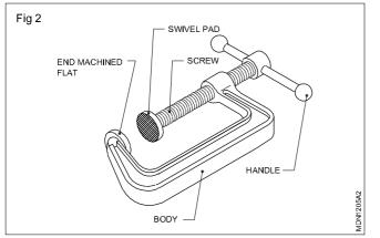
These clamps are used to hold work, on an angle plate or a drill press table, and also, for holding two or more workpieces together.
