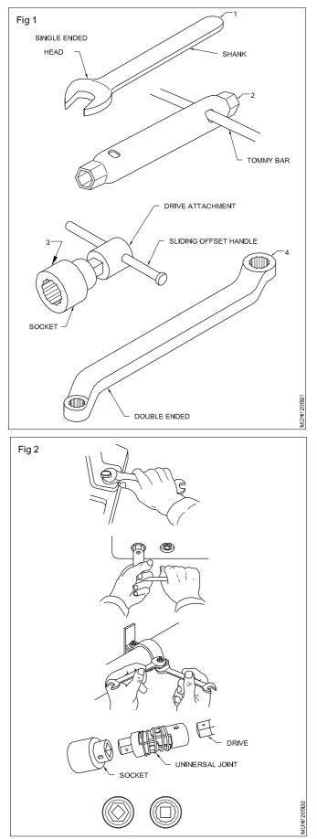
Use both hands as shown in the figure, when using tubular box spanners. (Fig. 2)
