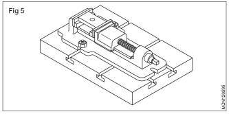
The toolmaker's vice is used for holding small work which required filing or drilling and for marking of small jobs on the surface plate. This vice is made of mild steel.
