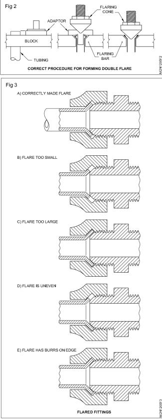
Flared tubing fittings : To attach a fitting to soft copper tubing, a flared type connection is generally used.
