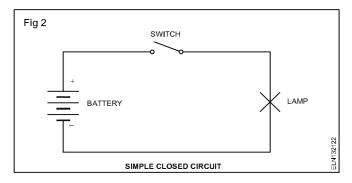
Flow of electric current is nothing but the flow of free electrons. Actually the electrons flow is from the negative terminal of the battery to the lamp and reaches back to the positive terminal of the battery.
