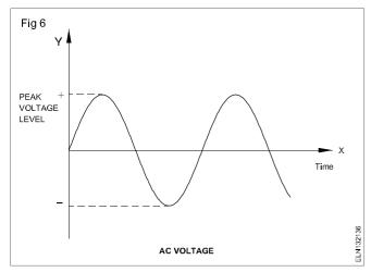
AC supply is expressed by the effective value of the voltage, and the number of times it changes in one second is known as frequency. Frequency is represented by 'F' and its unit is in Hertz(Hz).
