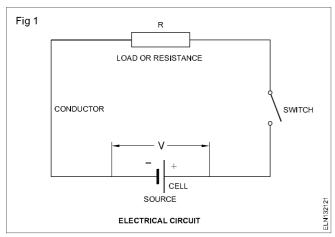
In addition to the above, the circuit may have insulators (PVC or rubber) to confine the current to the desired path, and a protection device (fuse 'F') to interrupt the circuit in case of malfunction of the circuit (excess current).
