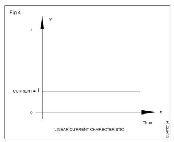
Thus direct current remains at the same value from the moment of switching on to the moment of switching off. (Direct current in common usage is known as DC current.)
