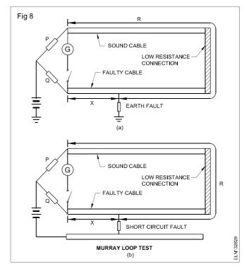
Where (R+X) is total loop resistance formed by the sound cable and the faulty cable. When the conductors have the same cross-sectional area and the same resistivity, the resistance are proportional to lengths. If  $I_1$  represents the length of the fault from the test end and 'l' is the length of each cable. Then
