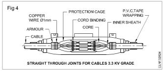
The cast iron protection boxes used up to 11 KV or moulds used for 1.1 KV joints in cast resin joints should conform to the relevant Indian Standard. Above 11 KV cast resin system is not yet standardized.
