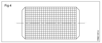
It is a knurling having a square shaped pattern. It is done by a set of rollers, one having straight teeth the other having teeth at right angles to the axis of knurl.
