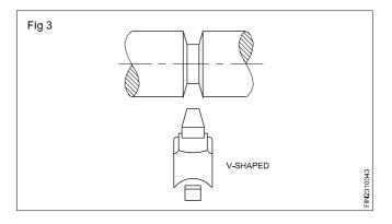
A tool bit ground to the desired angle is used to cut a shallow 'V' groove. Larger 'V' grooves such as those found on pulleys should be cut with the lathe compound rest to form each face of the groove individually.
