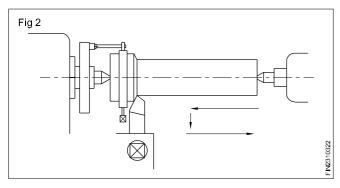
The spindle speed is calculated according to the material being turned, the tool material and the recommended cutting speed.
