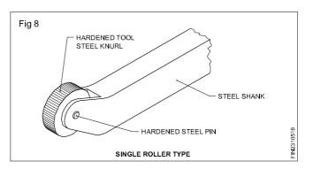
It has only one single roller which produces a straight lined pattern.
