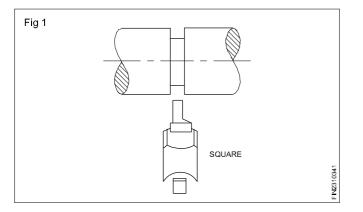
When a diameter is to be finished to size by grinding, a groove is generally cut against the shoulder to provide clearance for the grinding wheel and to ensure a square corner.
