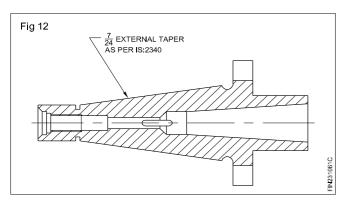
Spindle noses and arbors used on milling machines are usually provided with self-releasing tapers. The standard self-releasing taper is 7/24. This is a steep taper which helps in the correct location and release of the components in the assembly. This taper does not drive the mating component in the assembly. For the purpose of driving, additional features are provided.
