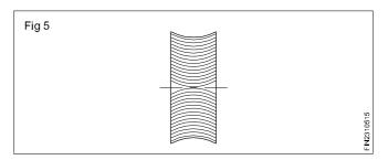
This is done by a convex knurl on a concave surface. This is done only by plunging the tool. The tool should not be moved longitudinally. The length of the knurling is limited to the width of the roller.
