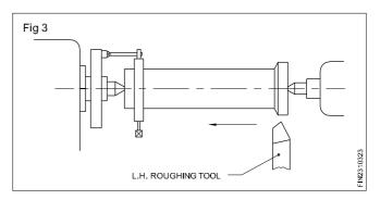
leaving sufficient metal for finishing. Surface finish and accuracy are not good. While rough turning, the spindle speed is less and the feed is more. A roughing tool or a knife tool is used.
