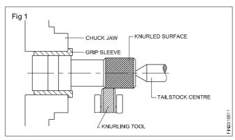
It is the operation of producing straight lined, diamond shaped pattern or cross lined pattern on a cylindrical external surface by pressing a tool called knurling tool. Knurling is not a cutting operation but it is a forming operation. Knurling is done at a slow spindle speed (1/3 the turning speed). However speed & feed given for knurling is to be divided according to the job material and the finish required.
