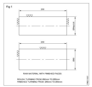
This operation involves removal of metal from the work and it has a cylinder for the full travel of the tool on the work, keeping the same diameter throughout the length.
