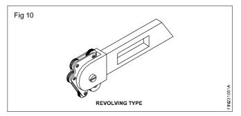
This tool-holder is also called a universal knurling toolholder. It is fitted with 3 pairs of rollers having coarse, medium and fine pitches. These are mounted on a revolving head which pivots on a hardened steel pin. It is also self-centering.
