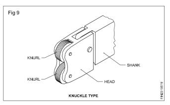
This tool holder has a set of two rollers of the same knurling pitch. The rollers may be of straight teeth or helical teeth. It is self-centering.
