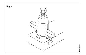
It consists of a circular tool post body and a pillar with a slot for accommodating the tool or tool-holder. Aring base, a rocker arm (boat piece) and a tool clamping screw complete the assembly of this type of tool post.
