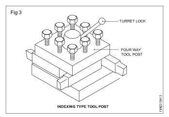
It is also called as square tool post or a four-way tool post. Four tools can be fixed in this type of tool posts, and any one can be brought into the operating position, and the square head is clamped with the help of the handle lever. By loosening the handle lever, the next tool can be indexed and brought in to the operating position. The indexing is manually.
