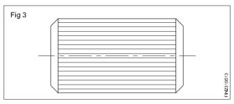
It is a knurling of straight lined pattern. This is done by using either a single roller or a double roller with straight teeth.
