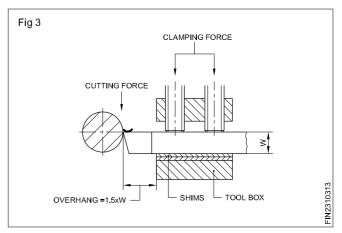
The unsupported length of the overhanging end of the turning tool should be kept to a minimum. As a rule, the overhanging length of tool is equal to the tool shank width x 1.5.
