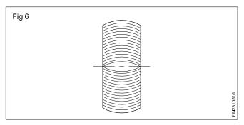
This is done by using a concave knurl on a convex surface. This is also done by plunging the tool.
