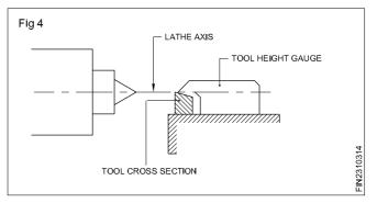
Remove or add shims and check the height when the tool is tightened by the centre screw.
