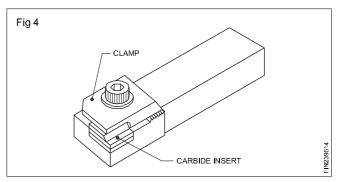
Carbide brazed tools when blunt or broken need grinding which is time consuming and expensive. Hence, they are used as throw-away inserts in mass production. Special tool-holders are needed and the carbide bits of rectangular, square or triangular shapes are clamped in the seating faces and machined on this type of special holders.
