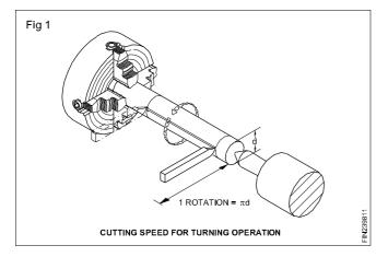
When a work of a diameter 'd' is turned in one revolution the length of the portion of work in contact with the tool is  $\pi$  x d. When the work is making 'n' rev/min, the length of the work in contact with the tool is  $\pi$  x D x n. This is converted into metres and expressed in a formula form as
