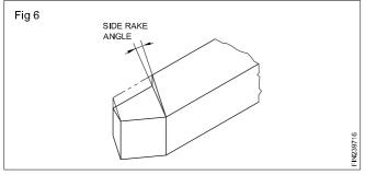
A side rake angle is the slope between the side of the cutting edge to the top face of the tool width wise. The slope is from the cutting edge to the rear side of the tool. It varies from  $0^{\circ}$  to  $20^{\circ}$ , according to the material to be machined.
