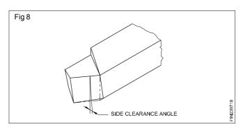
The clearance angle is the slope formed between the side cutting edge of the tool with a line perpendicular to the tool axis drawn downwards at the side cutting edge of the tool. The slope is from the top of the side cutting edge to the bottom face. This is also ground to prevent the tool from rubbing with the work, and allows only the cutting edge to contact the work during turning. The side clearance angle needs to be increased when the feed rate is increased.
