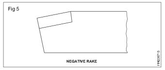
The top rake angle may be ground positive, negative or zero according to the material to be machined. When turning soft, ductile materials, which form curly chips, the positive top rake angle ground will be comparatively more than for turning hard brittle metals.
