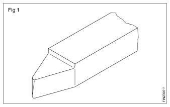
These are tools having their cutting edges ground on solid bits of square, rectangular and round cross-sections. Most of the lathe cutting tools are of the solid type, and high carbon steel and high speed steel tools are used. The length and cross-section of the tool depend upon the capacity of the machine, the type of tool post and the nature of the operation.
