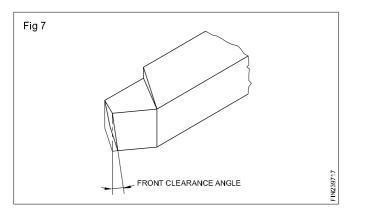
It is the slope between the front of the cutting edge to a line perpendicular to the axis of the tool drawn downwards which is known as the front clearance angle. The slope is from the top to the bottom of the tool, and permits only the cutting edge to contact the work, and avoids any rubbing action. If the clearance ground is more, it will weaken the cutting edge.
