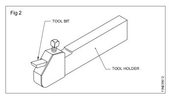
Solid high speed steel tools are costly; hence, they are sometimes used as inserted bits. These bits are small in sizes, and are inserted in the holes of the holder. These holders are held and clamped in the tool posts to carry out the operations. The disadvantage in this type of tools is that the rigidity of the tool is poor.
