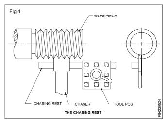
When chasing, the thread is cut slightly oversize, then trimmed down to size with the chaser; constantly check the thread with a thread ring gauge, if necessary.
