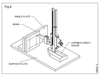
The vernier height gauge is used with the dial indicator to check hole location, pitch dimensions, concentricity and eccentricity.
