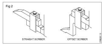
**Functional features of the vernier height gauge:** Vernier height gauges are used in conjunction with the surface plate. In order to move the main slide, both the locking screws of the slide and the finer adjusting slide have to be loosened. The main slide along with the chisel pointed scriber has to be set by hand, for an approximate height as required.
