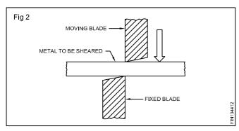
After a certain amount of plastic deformation, the cutting member begin to penetrate. The uncut metal work, harden at the edge (Fig 4).
