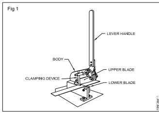
The lower blade of the hand lever shear is fixed (bottom blade) and the upper blade is pivoted at an angle.
