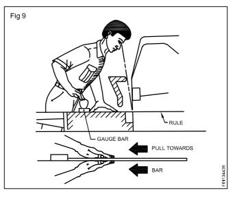
Cut the sheet metal to the size and shape as per marking
