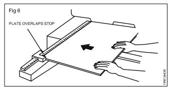
**Parallel setting of front gauge:** The front gauge is used when there is less overhang.
