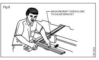
**Using scale on gauge brackets:** Where a machine is fitted with a graduated scale on the brackets, position gauge bar to the required dimension and fully tighten the nuts.
