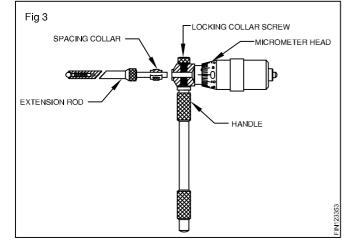
**Micrometer head:** It consists a sleeve, a thimble, an anvil and locking screw for extension rods.
