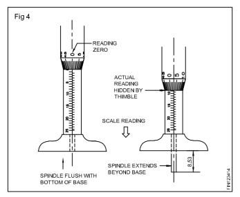
The advancement of the extension rod for one full turn of the thimble is one pitch which is 0.5 mm.
