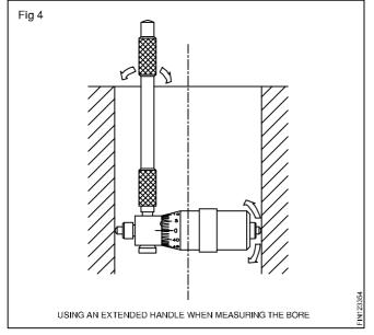
the top, another reading at the middle and the third reading at the bottom of the bore. If all the three readings are the same, then the surfaces of the bore are parallel. Any variation in the readings shows an error in the bore.
