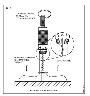
The graduations are numbered in the reverse direction, to that marked on an outside micrometer.
