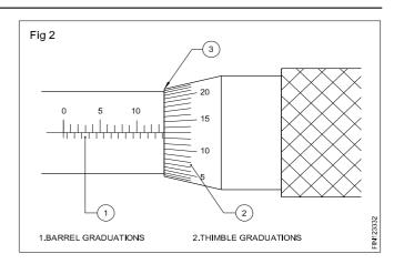
First note the minimum range of the outside micrometer. While measuring with a 50 to 75 mm micrometer, note it as 50 mm.
