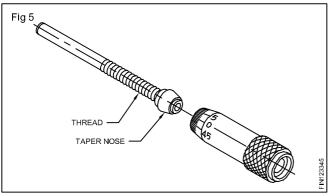
The taper nose is very accurately finished for axial alignment and it also permits postioning of the thimble in any required place during the adjustment of zero error.
