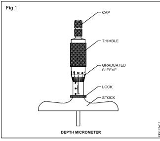
A set of extension rods is generally supplied. On each of them the range of sizes that can be measured with that rod, is engraved as 0-25, 25-50, 50-75, 75-100, 100-125 and 125-150.
