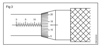
Constructional features of outside micrometer
