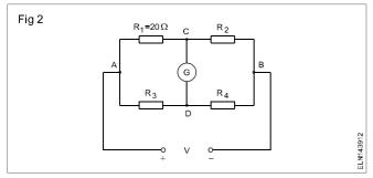
**Equal resistance ratio in parallel circuit**: One does not need equal resistances in the parallel circuits to obtain equal potential nodes. It suffices if the resistances are in the same ratio to each other.
