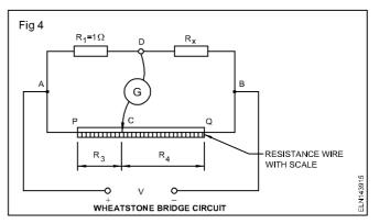
R<sub>1</sub> is a standard resistor, e.g. 1 ohm.
