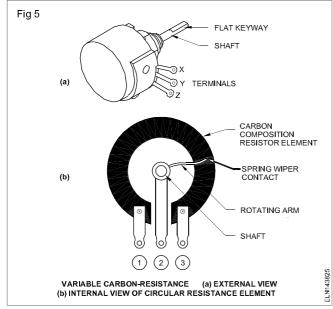
It is provided with 3 terminals as shown in Fig 5 and 6. They are available with carbon tracks (Fig 5) and wire wound (Fig 6) types. Trimmer potentio meters (or) resistor which can be adjusted with the help of a small screw drivers. (Fig 7).
