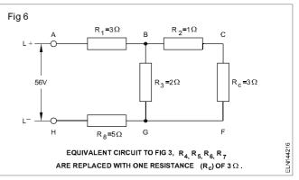
7 Combine  $R_2$  and  $R_c$  and call the equivalent resistance  $R_d$ .
