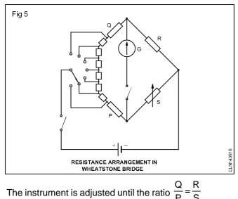
This is indicated by a zero reading on the galvanometer with its switch in the closed position.
