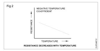
**Temperature coefficient of resistance (a) of a conductor:** Let a metallic conductor, having a resistance of  $R_0$  at 0°C, be heated to t°C and let its resistance at this temperature be  $R_t$ . Then, considering normal ranges of temperature, it is found that the increase in resistance depends:
