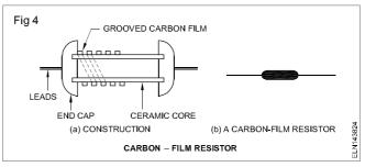
In this type, a thin layer of carbon film is deposited on the ceramic base/tube. A spiral groove is cut over the surface to increase the length of the foil by a specialised process.
