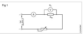
If the voltmeter resistance is not very large, compared with the resistor to be measured, the voltmeter current will be an appreciable fraction of the current I, measured by the ammeter, and a serious error may be introduced on this account.
