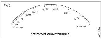
This ohmmeter has a non-linear scale because of the inverse relationship between resistance and current. This results in an expanded scale near the zero end and a crowded scale at the infinity end.
