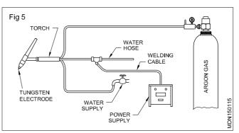
When the inert gas is replaced by carbon dioxide then it is called  $CO_2$  arc welding or metal active gas (MAG) arc welding.
