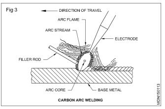
A separate filler rod is used since the carbon electrode is a non-metal and will not melt.
