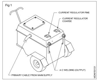
The A.C. main supply has high voltage - low ampere.
