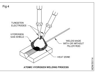
The welding job remains out of the welding circuit.
