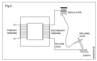
The A.C. welding machine cannot be operated without the A.C. main supply.
