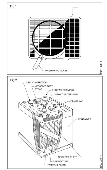
**Construction:** The automobile battery's plates are rectangular. They are made of lead. Antimony alloy is used to provide them strength.
