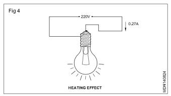
When a current is applied to a bulb filament (fine wire) it becomes white hot and thus produces light.
