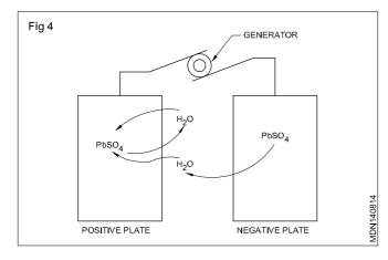
When the battery is charged (Fig 4) by passing current through a dynamo or charger in the opposite direction, the reverse chemical reaction takes place. The lead sulphate on one plate becomes lead peroxide (+ve plate). The lead sulphate on the other plate (-ve plate) becomes spongy lead and the electrolyte becomes more concentrated because of the increased amount of sulphuric acid.
