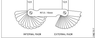
Each blade can be swung out of the holder separately, and has its size engraved on it. (Fig 8)
