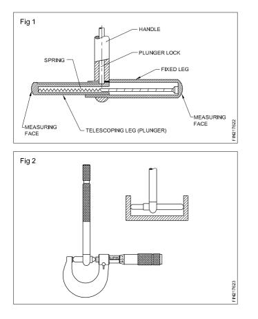
Telescopic gauges are available in a set of 6 nos, to measure holes from 8 mm to 150 mm. (as per MITUTOYO - Series 155)
