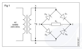
The operation of a bridge rectifier can be summarized in the following steps;
