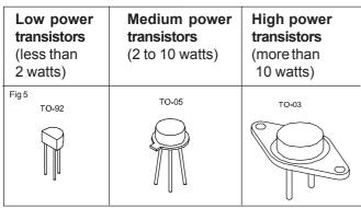
Low power transistors, also known as small signal amplifiers, are generally used at the first stage of amplification in which the strength of the signal to be amplified is low. For example, to amplify signals from a microphone, tape head, transducers etc.,
