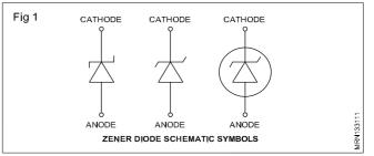
The difference between a rectifier diode and a zener diode are listed below;
