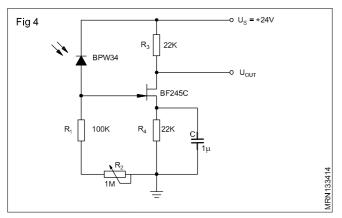
Circuit diagram of a simple Light controlled amplifier is shown in Fig 5. This circuit uses a single FET for amplifying the output of the photodiode connected in series with a resistor.
