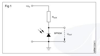
When no light is incident on the photodiode, a reverse current flows through the p-n junction, as it does in any normal semiconductor diode, but in photodiodes it is usually referred to as the "dark current"  $I_{Ro}$ .
