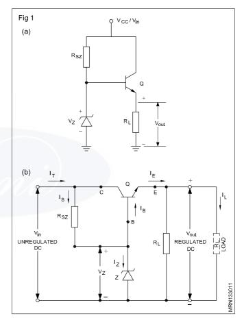
The voltage across the zener,  $V_z$  drives the base of the emitter follower. Therefore, the dc output voltage is bootstrapped to within one  $V_{BE}$  drop of the zener voltage. The regulated dc output voltage will be,
