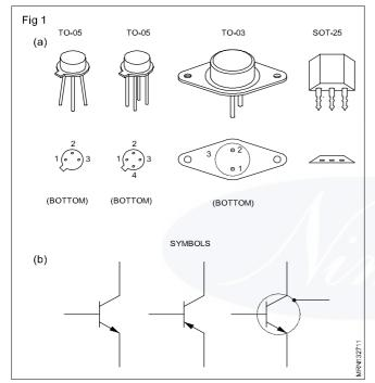
Transistors are mainly used for enlarging or amplifying small electric/electronic signals as shown in Fig 2. The circuit which uses transistors for amplifying is known as a transistor amplifier.
