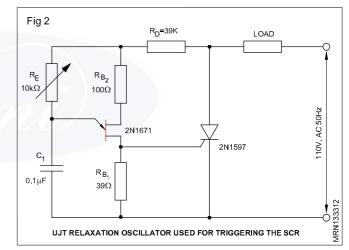
The low output impedance of the UJT (390hms) is ideal for driving the SCR, which has a relatively low input impedance from gate to cathode.
