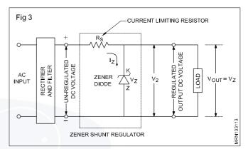
If the input DC voltage to the zener increases, as can be seen from its characteristics in Fig 2, the current  $I_z$  through the zener increases but the voltage across the zener remains the same due to avalanche effect. Because the zener voltage,  $V_z$  does not change, the output voltage  $V_{OUT}$ , does not change and so the voltage across the load is constant. Thus, the output is said to be regulated.
