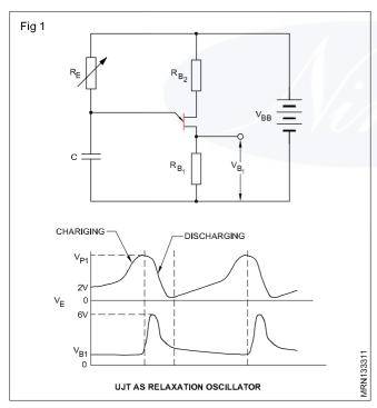
The negative - resistance portion of the UJT characteristic is used in the circuit shown in Fig 1 to develop a relaxation oscillator.
