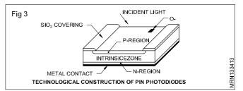
The advantages of PIN photodiodes are;
