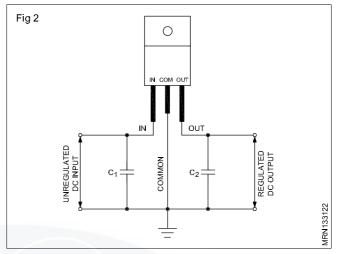
The capacitor  $C_2$  is used to improve the transient response of the regulated output voltage.  $C_2$  bypasses these transients produced during the ON/OFF time. Typical values of  $C_2$  range from 0.1  $\mu$ F to 10  $\mu$ F.
