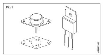
These ICs consists of all those components and even more in the small packages shown in Fig 1. These ICs, when used as voltage regulators, do not need extra components other than two small value capacitors as shown in Fig 2.
