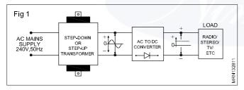
The transformer will step-down or step-up the mains AC to the required level. The stepped-up or stepped-down AC from the output of the transformer is then converted to DC using diodes making use of their unique unidirectional property.
