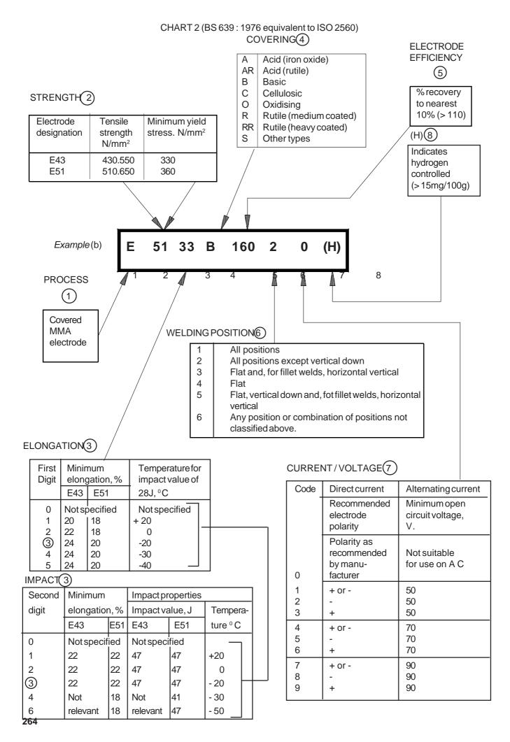
Example (1) Covered electrode for manual metal arc welding having a rutile covering of medium thickness and depositing weld metal with the following minimum mechanical properties. (BS 639)
