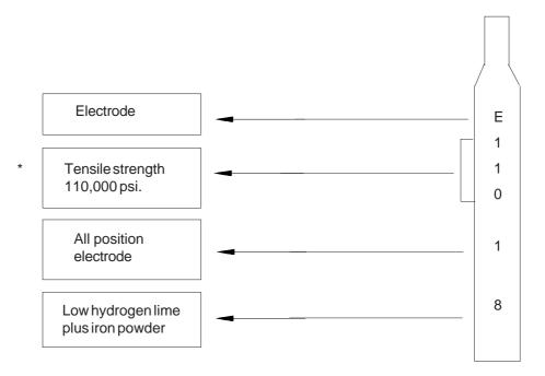
\* To get the tensile strength of the weld in p.s.i., the number given here should be multiplied by 1000.
