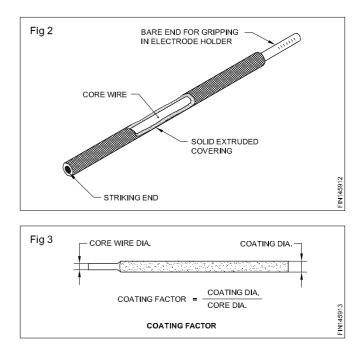
1.6 to 2.2 for **heavy coated**, and above 2.2 for super heavy coated electrodes.
