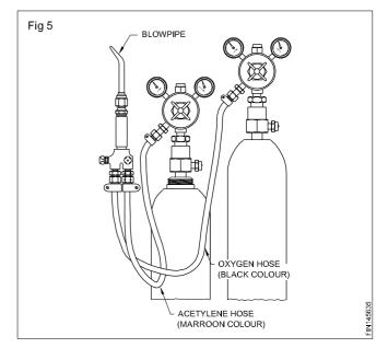
Rubber hoses are connected to regulators with the help of unions. These unions are right hand threaded for oxygen and left hand threaded for acetylene. Acetylene hose unions have a groove cut on the corners. (Fig 6)
