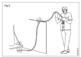
Inspect the rubber hose pipes periodically and replace the damaged ones.
