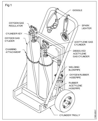
The basic equipments used to carry out gas welding are
