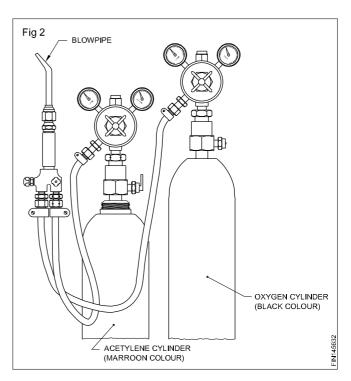
**Dissolved acetylene cylinders:** The acetylene gas used in gas welding is stored in steel bottles (cylinders) painted in maroon colour. The normal storing capacity of storing acetylene in dissolved state is 6m<sup>3</sup> with the pressure ranging between 15-16 kg/cm<sup>2</sup>.
