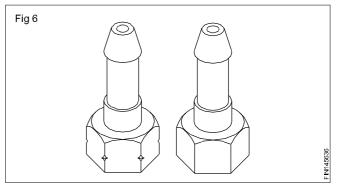
At the blowpipe end of the rubber hoses hose-protectors are fitted. The hose protectors are in the shape of a connecting union and have a non-return disc fitted inside to protect from flashback and backfire during welding. (Fig 7)
