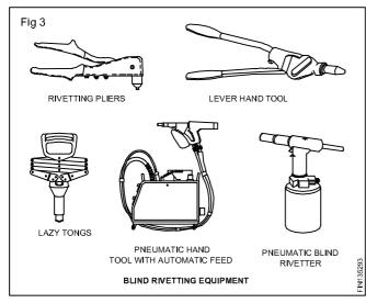
**Types of Blind or Pop rivets:** In setting a blind rivet, the body of the rivet is inserted into a hole and the mandrel is pulled deforming the tail which pulls and fixes the joint together. Blind rivets are available in many types and systems. Some of these are given here-under.
