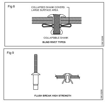
**Repetition blind riveting systems:** Rivet is loaded onto a mandrel which is placed into a pneumatic setting tool with a rivet in the ready position. This rivet is inserted into a preformed hole, the tool trigger is actuated, drawing the mandrel through the rivet, expanding the rivet tail. Sequence of rivet setting is shown in Fig 10.
