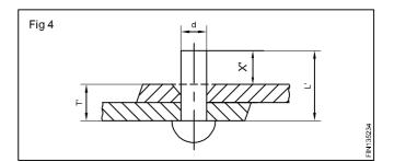
When he appropriate values of the rivet diameter and the length for the plate thickness are found out, choose the rivets with the standard size close to the calculated values.
