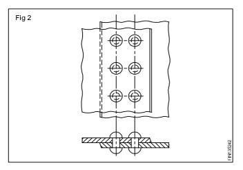
**Double riveted (Zigzag) lap joint:** This provides a stronger joint than a single lap joint. The rivets are placed either in a square formation or in a triangular formation. The square formation of rivet placement is called CHAIN riveting. The triangular formation of rivet placement is called zigzag riveting.(Fig 3)
