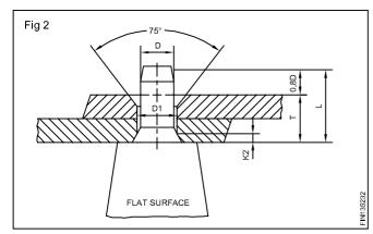
A formula generally used in the shop floor is length of snaphead rivets.
