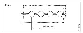
Too closely spaced rivets will tear the metal along the centre line of the rivets.
