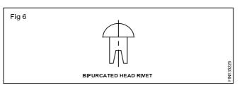
Selection of rivet size: The diameter of the rivet is calculated by using the formula D=(21/2 to 3) xT where T is total thickness
