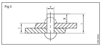
Therefore, the length of the rivet (L mm) to form a round head when the total thickness of the piled plates is T mm will be, as given below.
