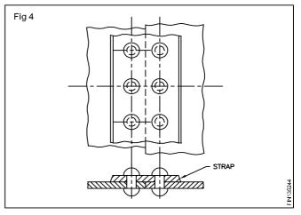
A separate piece of metal called STRAP is used to hold the edges of the components together.
