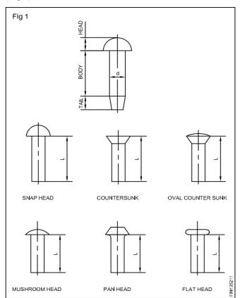
Rivets are cylindrical rods having heads of various shapes. They are used for assembling the parts of a workpiece together.
