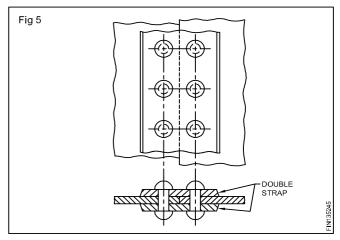
When single or double straps are used for riveted butt joints, the arrangement of rivets may be:
