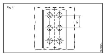
The distance will help to drive the rivets without interference.(Fig5)
