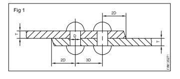
The space or distance from the edge of the metal to the centre of any rivet should be atleast twice the diameter of the rivet.
