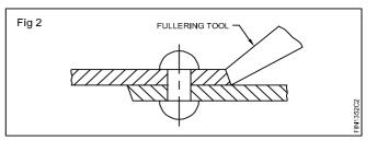
The whole surface of the edge of the first plate is tightly pressed on the second plate.
