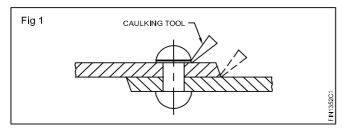
The edge of the rivet head is tightly pressed and expanded on the plate by a caulking tool which looks like a fattened cold chisel.
