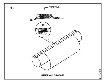
Hand Groover: The hand groover is made up of cast steel and is used to make external locked grooved joint.
