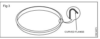
Make a round ring from the given G.I.wire to the required dia. (Fig 3)  $\,$
