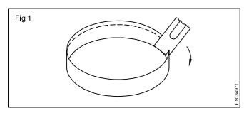
Flange the edge to be wired using a hatchet stake and a setting hammer, step by step upto  $90^{\circ}$ . (Fig 2) Then upset the flange to its half the width and make curve on the flange for wiring. (Fig 3)
