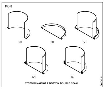
If the seam is not turned up, as in D, the seam is called paned down seam.
