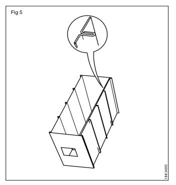
Strength and rigidly of the panel and the joint design is simple and cost effetive as shown in Fig.
