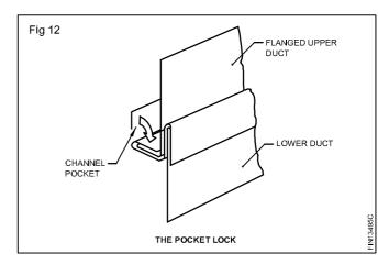
The upstanding fold of the channel is dressed down by hand, commonly at the time of installation.
