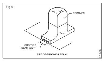
The hand groover is specified according to the size of the groove of the groover.
