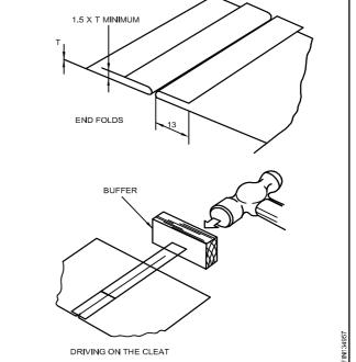
It is a good practice to insert a tongue into the end folds of the abutting cleat. An alternate is to bend the tongue and secure with blind the tongue and secure with blind rivets as shown in Fig 8. A similar corner finish may be done.
