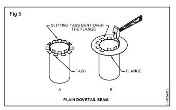
The straight tabs are bent over the part to be joined and the bent tabs act as stops. This seam may be made water tight by soldering around the joint.
