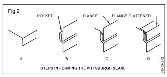
The advantage of the Pittsburgh seam is that the single lock can be turned on a curve and the pocket lock can be formed on a flat sheet and rolled to fit the curve as shown in Fig 3. If roll forming machine is not available in shop, Pittsburgh seam is formed on the brake.
