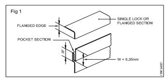
Single lock can be turned on the curve and pocket lock to be formed on a flat sheet and then rolled to fit the curve.
