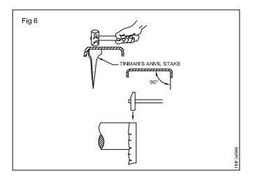
Position the cylinder as in Figure 1 and strike the metal using the flat face of the finishing hammer.
