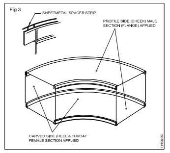
**Snap lock seam:** Snap lock seam is as role formed seam and is machine similar to pittsburgh lock seam. (Fig 3)
