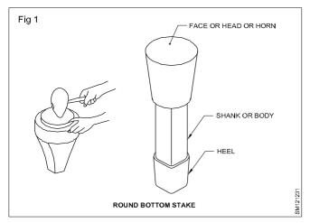
**Round bottom stake** (Fig 1): It has a round and a concave face head. It is used for hollowing the sheet.
