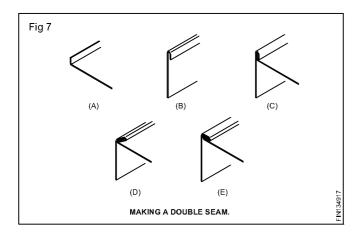
The other type is used to fasten bottoms to cylindrically shaped jobs such as pails, tanks etc.
