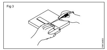
Try squares are specified according to the length of the blade i.e. 100 mm, 150, 200 mm.
