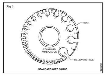
Gauge number is stamped on one side of each slot and on the other side, the decimal part of an inch is stamped to show the thickness of the sheet and the diameter of the wire.
