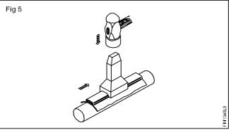
The joint is locked working along the joint in stages.
