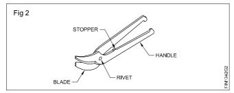
**Specification:** Bend snips are specified by their overall length. Bend snips are available in 150, 200, 300 and 400 mm length.
