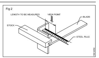
For maintaining the accuracy of the steel rule, it is important to see to it that its edges and surfaces are protected from damage and rust.
