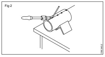
**Electric soldering copper bit:** The bit of the electric soldering iron is heated by an element. This type is preferred, if current is available because it maintains uniform heat. Electric soldering irons are available for different voltages and are usually supplied with a number of interchangeable tips. They can be made quite small and are generally used on electrical or radio assembly work. (Fig 3)
