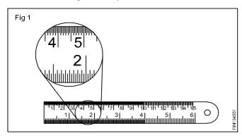
For accurate reading it is necessary to read vertically to avoid errors arising out of parallax. (Fig 2)
