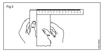
To mark lines at 90° to the edges of a workpiece. (Fig 3)
