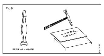
**Specification:** The sheet metal hammers are specified by the Type of pane and the weight of the hammer.
