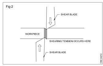
**Cutting edge of the blade and clearance**: Clearance between the blades should be free but without gap. For straight snips, cutting angle is 87°.
