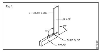
The accuracy of measurement by a try-square is about 0.002 mm per 10 mm length, which is accurate enough for most workshop purpose. The try-square has a blade with parallel surfaces. This blade is fixed to the stock at 90°. Burr slot is provided on the stock at meeting point of blade to accommodate the burr, if present on the component, to avoid inaccuracy in measuring squareness.
