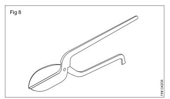
**Rohdes shears:** Its one handle is shorter in length as compared with the other handle as shown in Fig.9.
