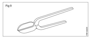
The short handle is to be pressed by the right leg of the worker and the other handle should be held by the right hand. It is used to cut lengthy sheets.
