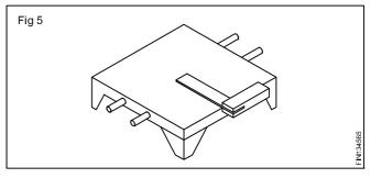
If the two marked lines are in one line as shown in Fig 6. Trysquare blade is 90° to the stock and it is correct.
