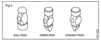
**Cheek:** The cheek is the middle portion of the head. The weight of the hammer is stamped here. This portion of the hammer head is left soft.
