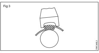
Then the groover is placed over the closed end of the joint. The groover is positioned at a very slight angle. The edge of the joint acts as a guide to position the groover.
