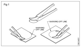
Parts of the bend snips are shown in fig 2. The blades of the bend snips are curved. (Fig 2)
