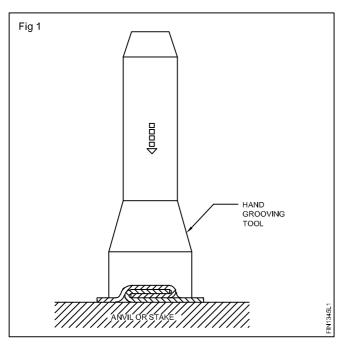
The end of the tool is recessed to fit over the lock making the grooved seams. (Fig 2)
