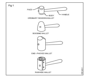
Avoid using the mallet as hammer for doing chipping and to drive nails and work on the sharp corners.
