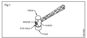
The handle is fixed in the eye hole of the hammer at right angle to the head.
