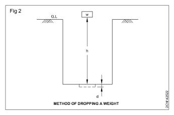
In this method a substance of known -weight is dropped from a known-height as shown in figure. The depth of impression made by the weight on the soil is noted.
