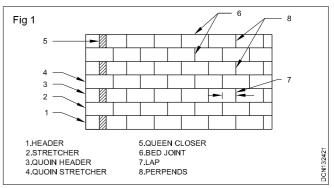
**Stretcher** : A brick laid with its length parallel to the face of the wall
