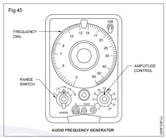
under ordinary test conditions. For any given setting of the amplitude control, the output signal is stable as the frequency is varied and remains undistorted within the tolerances below.
