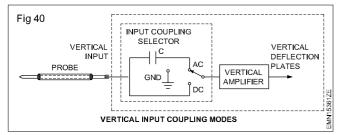
The DC coupling mode is used in majority of oscilloscope measurements whether it is measuring DC amplitudes or seeing logic low and high levels over analysing transient and repetitive AC waveforms over the specified bandwidth of the oscilloscope. However, when it comes to measuring only the amplitude of a certain DC voltage with no intention of analysing the quality of DC or looking for presence of any noise spikes, the oscilloscope in the DC coupling mode does the job.
