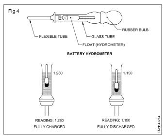
The importance of specific gravity can be seen from the fact that the open circuit voltage(V) of lead-acid battery is approximately given by,
