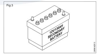
A battery may consist of two or more number of cells. The battery shown in Fig 3 has six cells of 2V each. These cells are connected in series to give 12V at battery terminals.
