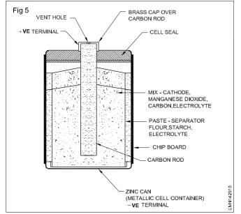
The two electrodes of dry cells are brought out and are available as +ve and -ve terminals of the cell. Usually the metallic cell container serves as the -ve of the cell as
