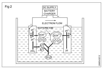
water is removed from the electrolyte solution. As the electrolyte returns to its normal strength of sulphuric acid (27%) and the plates return to their original form of lead peroxide and spongy lead, the voltage across the electrodes returns to its nominal value of 2.2 V. The chemical action involved during charging can be represented by the following equation;
