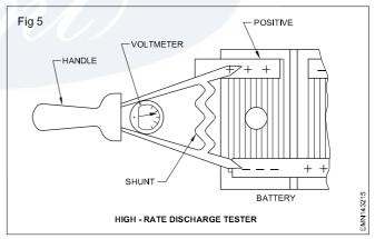
The two terminal prods are pressed on to the terminals of a cell for testing. For fully charged cell the meter pointer points in the range of *full charge* on the meter scale. A sulphated old cell will show the discharge reading. The meter is having three colours red, yellow and green; red for fully discharged, yellow for half charged and green for fully charged condition of the cell respectively.
