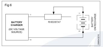
In constant current charging, the output DC voltage of the charger will be generally twice the nominal voltage of the battery to be charged. But, the charging current is controlled by varying the rheostat connected in series with the battery. For example, to charge a 12 V battery, the DC voltage source can be 24 V, but the charging current will be kept controlled say, 1 ampere with the help of the rheostat.
