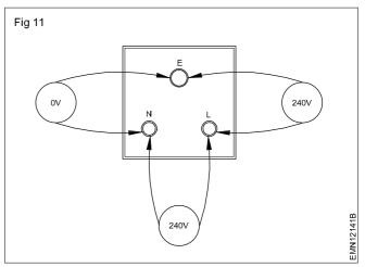
Any defect either in mains supply or in the wiring of the socket or in the equipment connected to any other 3 pin
