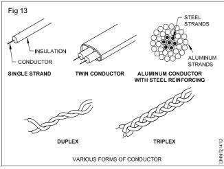
Conductors form an unbroken line carrying electricity from the generating plant to the point where it is used. Conductors are usually made of copper and aluminium.
