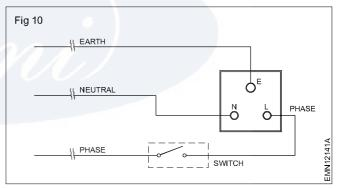
Referring to the Fig 10, when the switch is put ON, the voltages across the three points in a 3 pin socket should be as shown in Fig 11.
