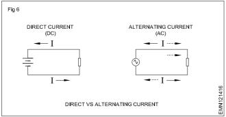
Whereas the familiar battery symbol is used as a generic symbol for any DC voltage source, the circle with the wavy line inside is the generic symbol for any AC voltage source.
