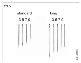
The needle has to be able to penetrate the material being sewn, without damaging it, by pushing the yarns aside. Solid materials, such as leather or plastic, will be holed. Sewing machine needles of various types are available. according to the application.
