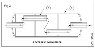
(3) of the muffler. Exhaust gases flow in a zigzag way, thus reducing the sound, by travelling through a longer length.
