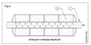
wool (2) is filled in between the perforated tube and the muffler housing, which acts as a sound absorbent.
