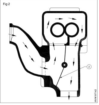
the exhaust gases are directly sent to the muffler.
