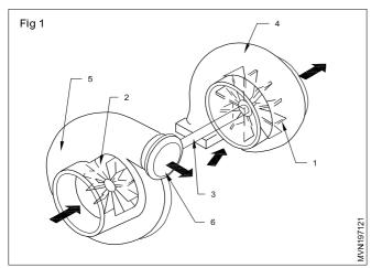
A turbocharger is mounted on the exhaust manifold. It has a turbine wheel (1) and a compressor wheel (2) on the same shaft (3). Exhaust gases enter in turbine housing (4) and rotate the turbine wheel (1). Compressor housing's (5) inlet is connected to the air cleaner and compressed air is discharged to inlet manifold through the outlet (6).
