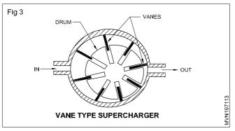
on decreasing in volume and increasing in pressure as in reaches the outlet.
