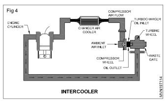
The intercooler (Fig 4) is an additional component that looks like a radiator, except that air passes through the inside as well as the outside of the intercooler. The intake air passes through sealed passageways inside the cooler, while cooler air from outside is blown across fins by the engine cooling fan.
