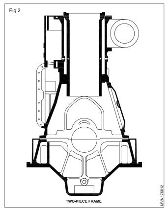
This portion where the crankshaft is fixed is known as the crankcase. In the cylinder block passages are provided for the camshaft and camshaft bearing, push rods, tappets etc.
