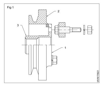
As the crankshaft speeds up or slows down, the damper flywheel has a dragging effect. This effect slightly flexes the rubber insert (3) which tends to hold the pulley and crankshaft to a constant speed. This tends to take on the twist and untwist action and torsional vibrations of the crankshaft.
