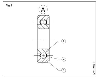
Ball bearings consist of an inner race (2), outer race (3) and balls (4). These bearings are used in the gearbox.
