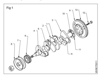
The front end of the crankshaft carries the gear or sprocket (6) to drive the cam shaft. A vibration damper (7) and a fan belt pulley (8) are fitted in front. The pulley (8) drives the water pump, engine fan and generator/alternator, through a fan belt.
