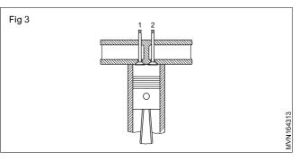
In the 'I' head the inlet (1) and exhaust valves (2) are located on one side of the cylinder head. The valves are operated by a single camshaft through the tappet, push-rod and rocker arm mechanism. (Eg. Ambassador, Ashok Leyland).
