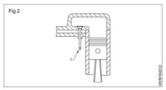
In the 'L' head, the inlet and exhaust valves (1) are located on one side of the cylinder block and the valves are operated by a single camshaft through the tappet directly. (Eg. Dodge)
