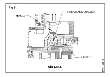
When the piston moves down on its working or power stroke, air pressure is at its maximum in the cell and pressure in the main combustion chamber starts to fall down. The higher pressure in the air cell causes its air to expand and blow out into the main chamber. Thus an additional turbulence is created and complete combustion of fuel charge is ensured.
