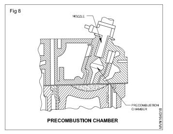
Pressure increases and the fuel droplets are forced through the small holes into the main cylinder, resulting in a very good mix of the fuel and air. The bulk of the combustion actually takes place in the main cylinder. This type of combustion chamber has multi-fuel capability because the temperature of the prechamber vaporizes the fuel before the main combustion event occurs.
