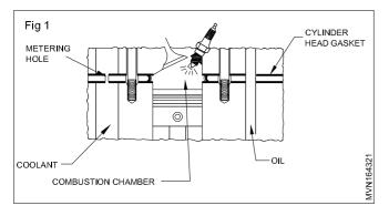
The head gasket must seal the combustion, pressures up to 1,000 psi (689.5 kPa) in gasoline engines and 2,700 psi (1,862 kPa) in turbocharged diesel engines. In addition, the head gasket must withstand combustion temperatures that are in excess of  $2,000^{\circ}F(1,100^{\circ}C)$ .
