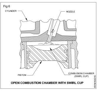
The deep cut-out swirl cup on the piston crown is being widely used.
