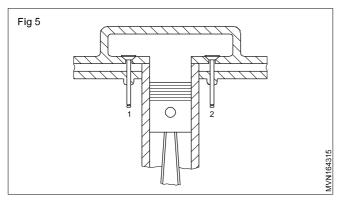
In the 'T' head, inlet valves (1) are located on one side of the cylinder block and the exhaust valves (2) are located on the other side of the cylinder block. Two camshafts are used to operate the valves, one for inlet and the other for exhaust. The valves are operated by the tappet directly. (Eg. Ford)
