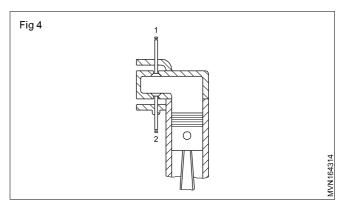
In the 'F' head, the inlet valves (1) are located on one side of the cylinder head and the exhaust valves (2) are located on the other side of the cylinder block. The valves are operated by a single camshaft. The inlet valves are operated by the tappet, push-road and rocker arm mechanism. The exhaust valves are operated by the tappet directly. (Eg.Mahindra & Mahindra jeep)
