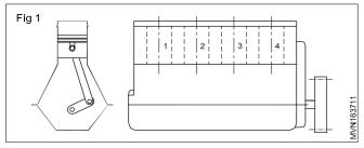
In this type, the cylinders are arranged in one line. The length of the crankshaft is longer than that of the other types of engines, and hence a limited number of cylinders are used. Better balancing and more uniform torque is obtained in this type.
