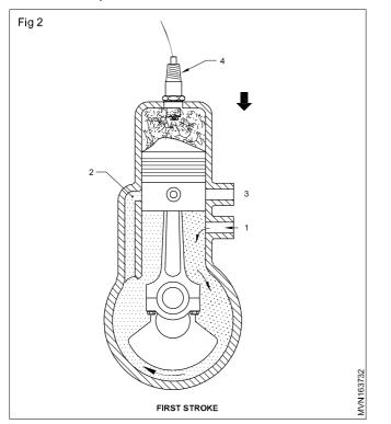
Further downward movement of the piston opens the transfer port and allows the partially compressed mixture, received during the previous stroke, to reach the combustion chamber from the crankcase.
