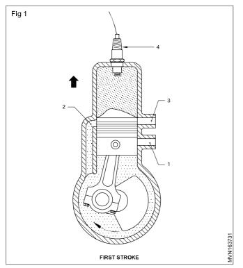
partial vacuum inside the crank-case below the piston, and the air/fuel mixture is drawn into the crank-case through the inlet port (I). The exhaust and transfer ports remain closed during the operation of the upward stroke and the charge which reached above the piston during the previous stroke is compressed.
