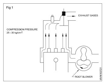
As the piston moves up from BDC to TDC the scavenging port and outlet valve closed. The piston compresses the fresh air to the compression chamber. The air temperature increases intensively.
