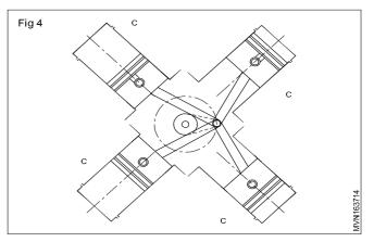
In this type, the cylinders are arranged radially. This type of engine is shorter, lighter and more rigid. Since it is rigid, a higher engine speed is possible and a higher combustion pressure can be obtained. This leads to high fuel efficiency. The radial type engines are used mostly in aeroplanes.
