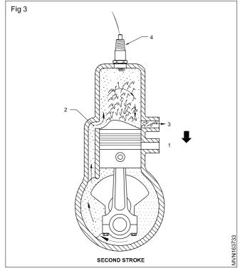
In this type of engine the compression ratio is low.
