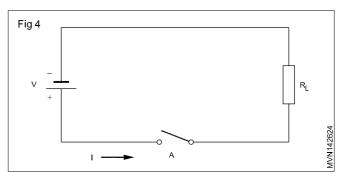
**Short circuit**: A short circuit will occur when two terminals of the same circuit touch each other. A short circuit may also occur if the insulation between the two cores of the cable are defective. This results in a lower resistance. This causes a large current to flow which can become a hazard.
