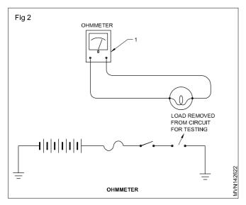
An ohmmeter (1) is also known as resistance meter.
