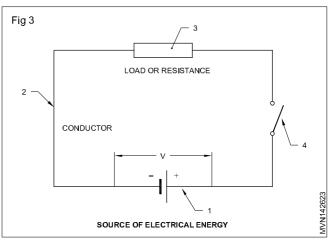
**Open circuit** (Fig 4): In an open circuit, an infinite resistance is provided, most of the time by the open switch (A). Therefore no current can flow.
