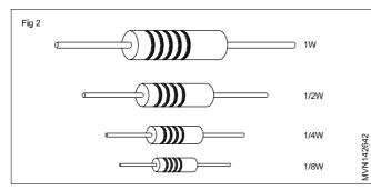
Selection of a particular type of resistor is possible based on its physical appearance. Table 1 at the end of this lesson illustrates the physical appearance of most commonly used fixed value resistors. The resistance value of a resistor will generally be printed on the body of the resistor either directly in ohms as shown in Fig 2a or using a typographic code as shown in Fig 2b or using a colour code as shown in Fig 2c.
