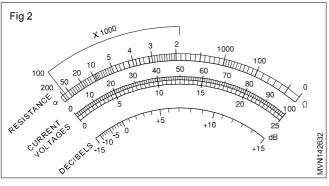
The scale for resistance measurement is non-linear. That is, the divisions between zero and infinity ( $\infty$ ) are not equally spaced. As you move from zero to the left across the scale, the division become closer together.
