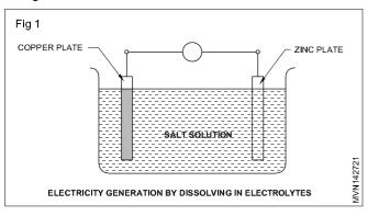
Copper and Zinc in salt solution is one combination
