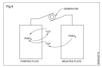
**Maintenance of battery:** Batteries are expensive items to replace. They should be serviced regularly as recommended by the manufacturer. If maintained properly, they
