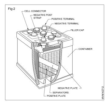
The group of plates, which are connected to the positive terminal of the cell, consists of grids filled with a paste of lead peroxide. This lead is brown in colour. The group of plates, which are connected to the negative terminal of the cell, consists of grids filled with metalic lead which is spongy in nature. This lead is dull grey in colour.
