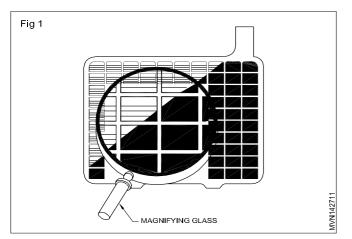
**Construction:** The automobile battery's plates are rectangular. They are made of lead. Antimony alloy is used to provide them strength.
