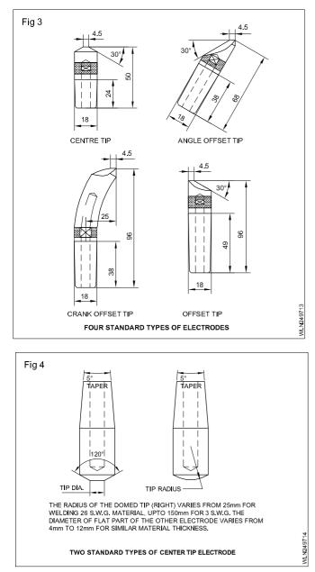
Regular spot welding leaves slight depressions on the metal. These depressions are minimized by the use of larger sized electrode tips and by inserting 1.6 mm copper sheets between the electrode and the job.
