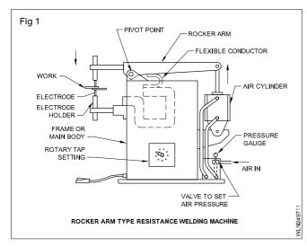
**1 The frame:** It is the main body of the machine which differs in size and shape for the stationary and portable types.
