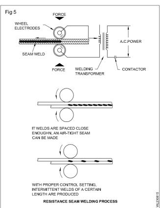
As the electrodes revolve, the current is automatically turned 'on' and 'off' at intervals corresponding to the speed at which the parts are set to move. With proper control, it is possible to obtain airtight seams suitable for containers, water heaters, fuel tanks etc.
