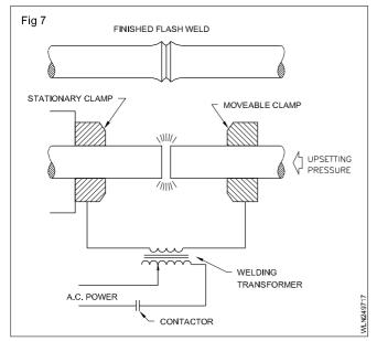
The ends of two metal pieces are moved towards and away from each other until an arc is established. The flashing action across the gap melts the metal, and as the two molten ends are forced together, fusion takes place. The current is cut off just before the heavy pressure is applied through the movable clamp. Flash butt welding is used to butt-weld plates, bars, rods, tubing and extruded sections. It is not generally recommended for welding cast iron, lead and zinc alloys.
