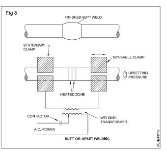
This process differs from flash butt welding in that constant pressure is applied during the heat process which eliminates flashing. The heat generated at the point of contact results from resistance. The operation and control of the butt welding process is almost identical to that of flash butt welding.
