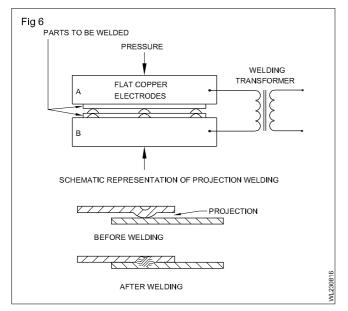
Either single or a multitude of projections can be welded simultaneously.
