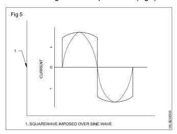
With the advent of modern electricity AC welding machines can now be produced with a wave form called Square Wave. The square wave has the benefit of a lot more control and each side of the wave can be, in some cases, controlled to give a more cleaning half of the welding cycle, or more penetration.
