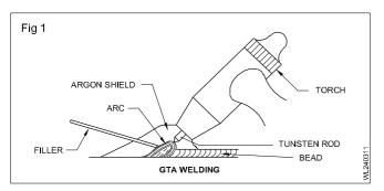
The GTAW process can produce temperatures of up to 3000° F. The torch contributes heat only to the workpiece. If filler metal is required to make the weld, it may be added manually in the same manner as it is added in the oxyacetylene welding process, or in other situations may be added using a cold wire feeder.
