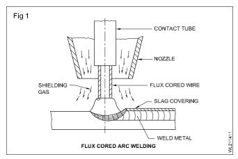
There are two major versions of the process, namely self shielded type (in which the flux performs all the functions of shielding) and the 'gas shielded type', which requires additional gas shielding.
