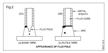
**Classification of flux cored wires:** The basic functions of the flux contained within the tubular wire include providing protective slag on the weld bead, introducing the required alloying elements and deoxygenerators into the weld pool and providing stability to the arc, besides producing the required shielding medium to protect the arc and weld pool.
