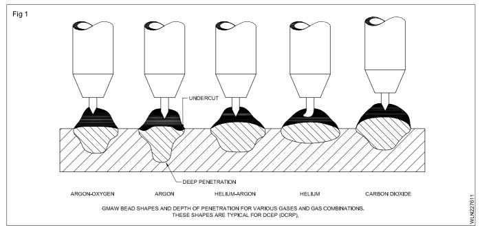
Argon used with the gas metal arc spray transfer process tends to produce deeper penetration through the center line of the bead. Spray transfer occurs more easily in argon than in helium.
