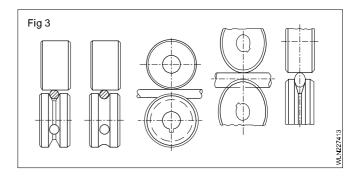
iii) all guides must be as close as possible to the drive roller to prevent the possibility of the wire bunching up.
