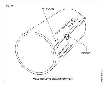
**Preheat:** Surface of the base metal is raised to a fairly high temperature 750°C (peacock neck blue colour) before the actual welding is started.
