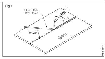
Ensure complete removal of all traces of flux because the residual flux will react and reduce the strength of the joint.
