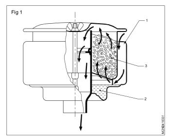
The atmospheric air enters the air cleaner through the side passage (1) and strikes on the surface of the oil (2). Heavy dust particles are absorbed by the oil. The partially filtered air, along with oil particles, moves upward through the filter element (3). Fine particles and oil particles are collected by the filtering element (3). Cleaned air then passes through the passage to the inlet manifold.
