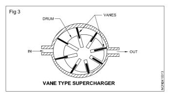
The roots syoercharger is simpler in construction and requries least mainteneace. It ha scomparatively ling life. It works well even at lower speed ranges. Centrifugal type supercharger has poor working charateristics at lower speeds. Vane type supercharger has the problem of wear of vane tips.
