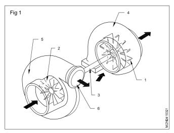
A turbocharger is mounted on the exhaust manifold. It has a turbine wheel (1) and a compressor wheel (2) on the same shaft (3). Exhaust gases enter in turbine housing (4) and rotate the turbine wheel (1). Compressor housing's (5) inlet is connected to the air cleaner and compressed air is discharged to inlet manifold through the outlet (6).
