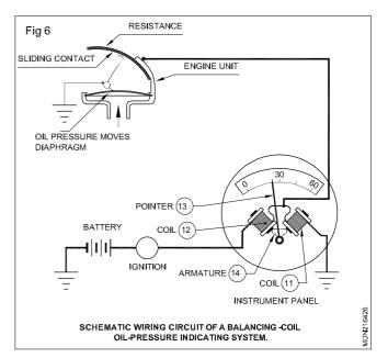
The right hand coil of the dash unit becomes magnetically stronger than the left hand coil.
